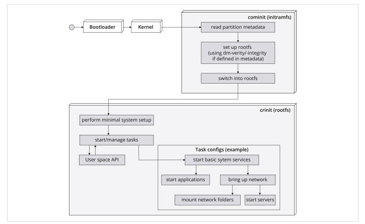
Figure 1: Flow diagram of a Linux bootup
