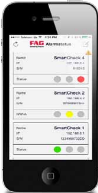
The alarm status of the FAG SmartCheck system can also be called up using mobile devices.
