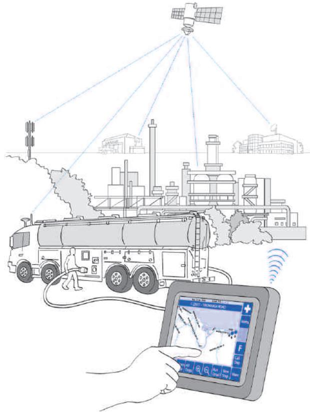
For liquid-transporting road tankers emlix has developed a telematics and logistics solution: a Linux system with control and operation applications is connected with the business IT of the fleet operator using the mobile telephone network. The system consists of a unit in the driver's cab and the control and operation system on the semi-trailer. Using these devices the loading and unloading procedures and the taking of samples can be controlled, and the operational security can be monitored.
